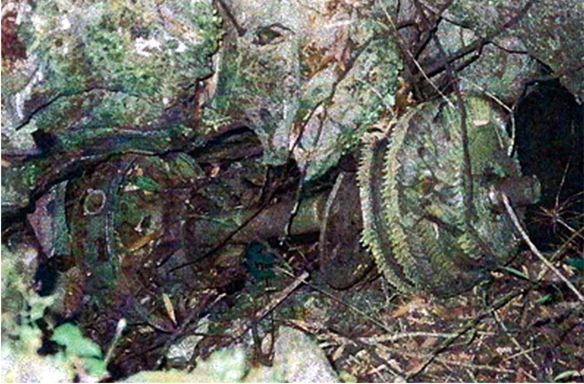
Landing gear strut and an engine drive shaft are two of the few heavy pieces of aircraft remains that were not carted off by the natives. (JPAC photo)
